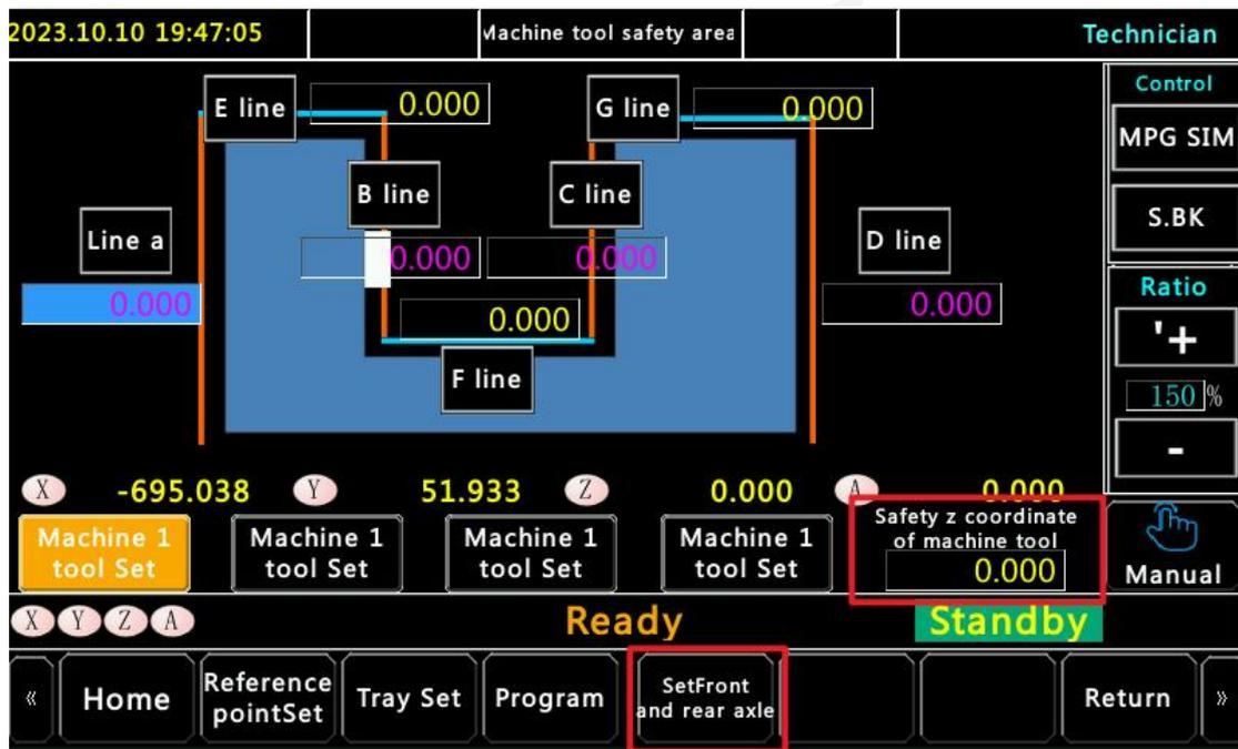
Step 2: Move the robotic arm above line E of the lathe and click the "E Line" button. The current Z-axis coordinate of the arm will be immediately filled in the field and take effect. Repeat this step, jog the robotic arm to move its position above other lines, and proceed with the point setting and modification of the safety area.
