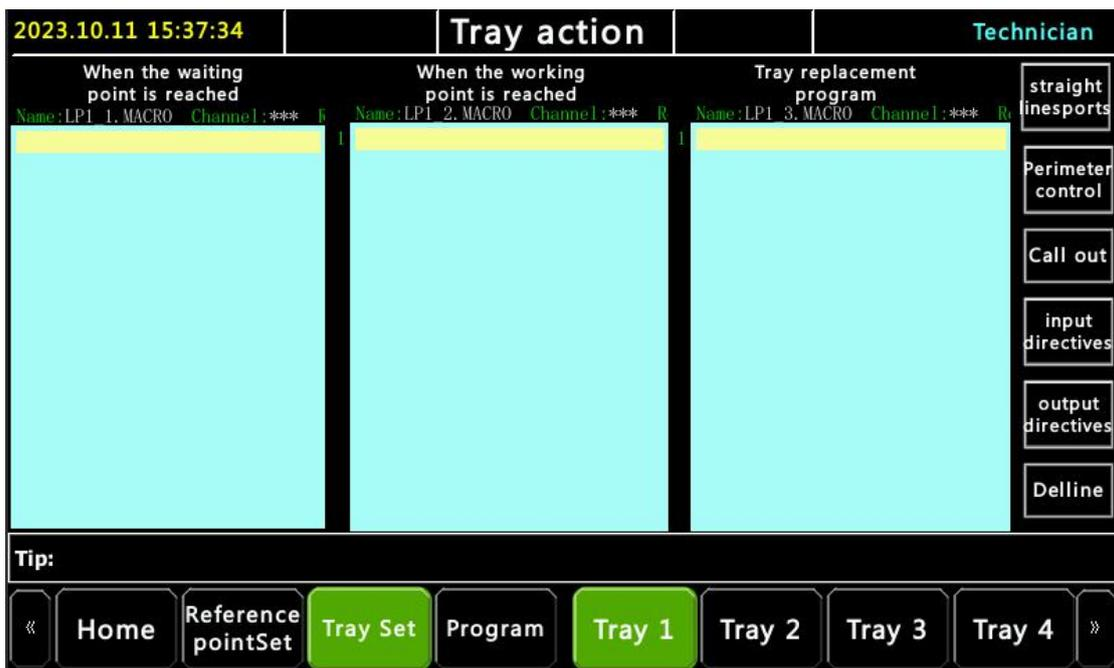
1. At Wait Point: Program executed when the robot reaches the waiting point.
