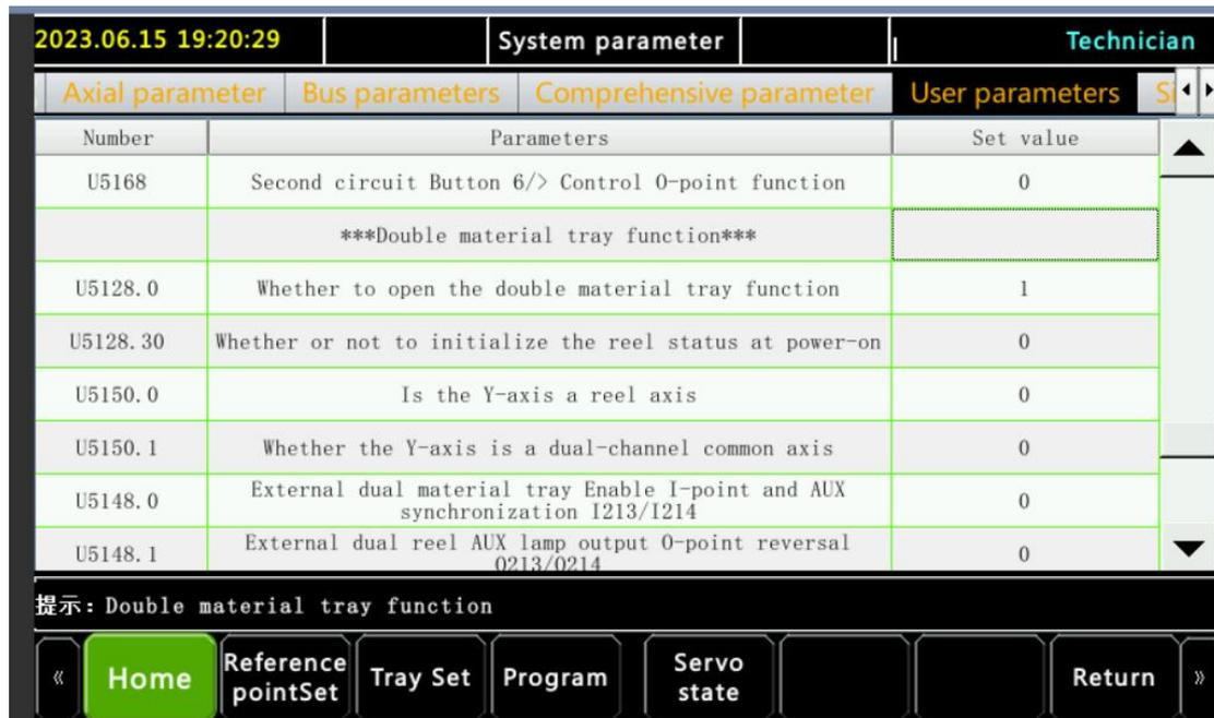
B. Step 2: Basic Parameter Setup in Tray Interface
