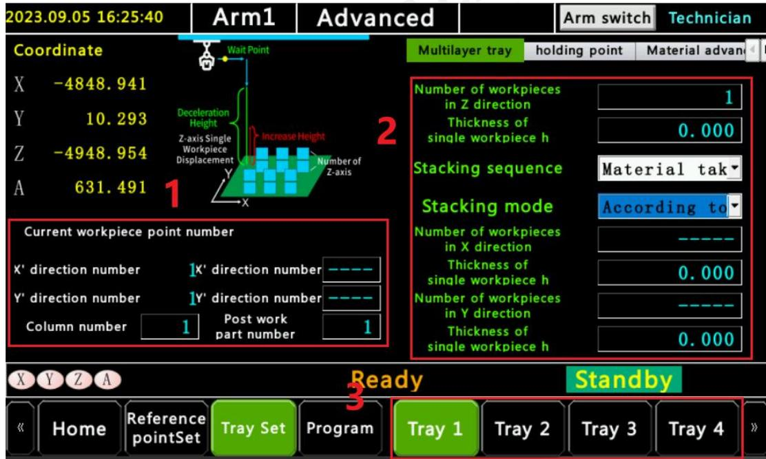
1. Workpiece Number Display Area: Displays the current target workpiece number, including position and layer.
