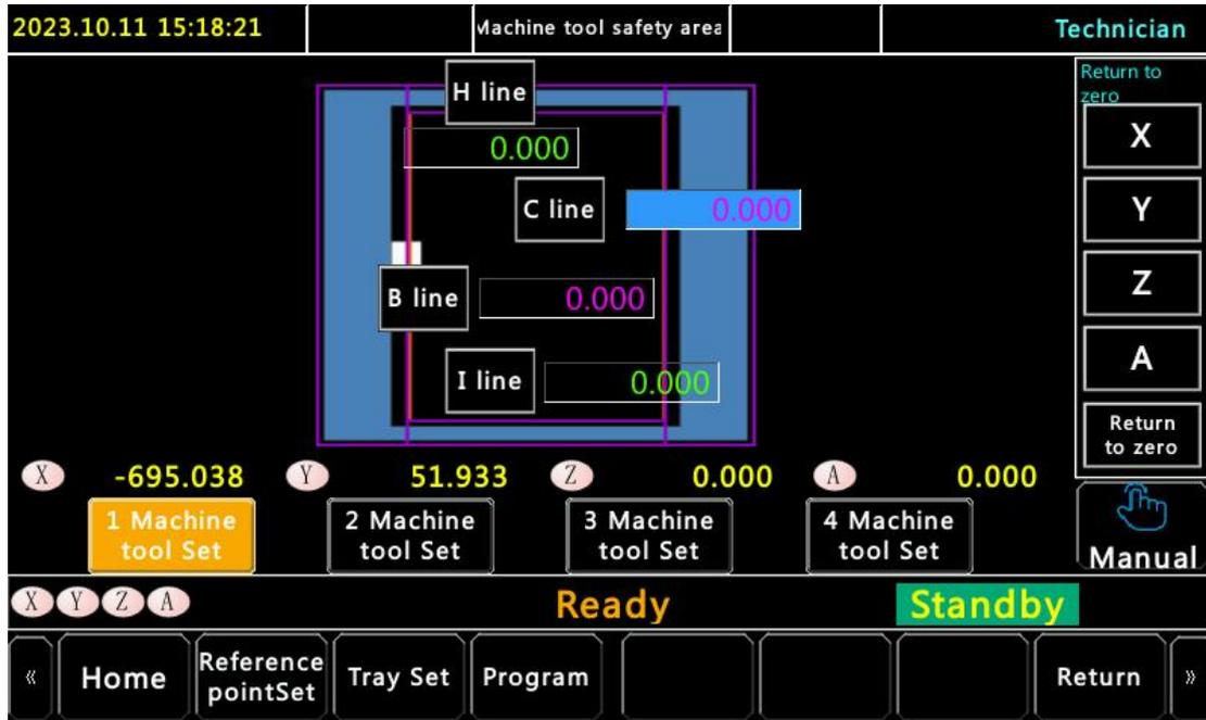
Step 5: Note that there are four sets of lathe numbers for coordinate setting. After completing the coordinate setting, return to the main interface and enable the corresponding lathe number.
